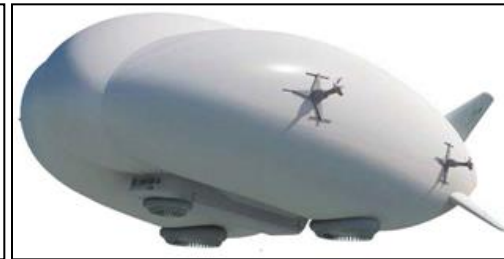
Buoyancy Thrust Vectoring Aerodynamic Lift (>40% AUW)
